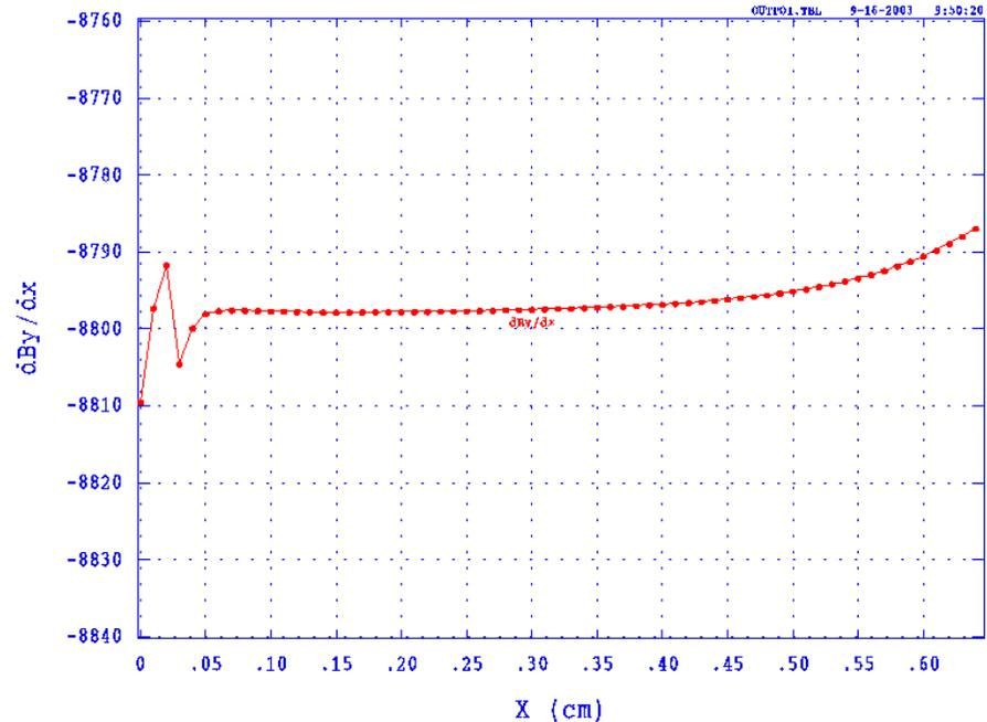
**The field gradient error is less than 0.2% within bore radius.**
