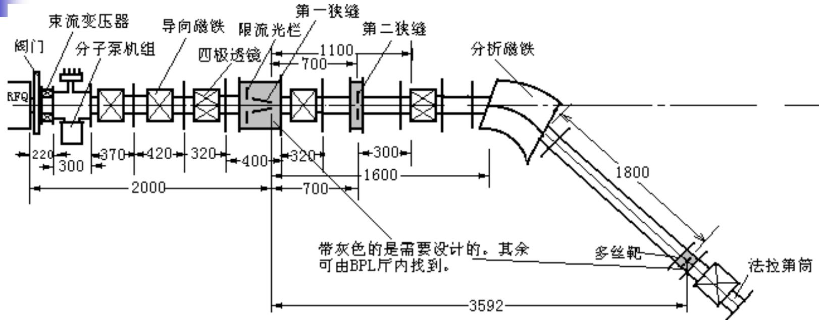
MEBT for the beam diagnostics is designed.
