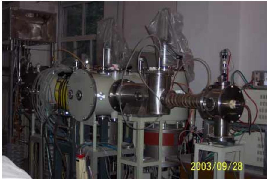
The Kicker in the LEBT will soon be setup for beam test.
