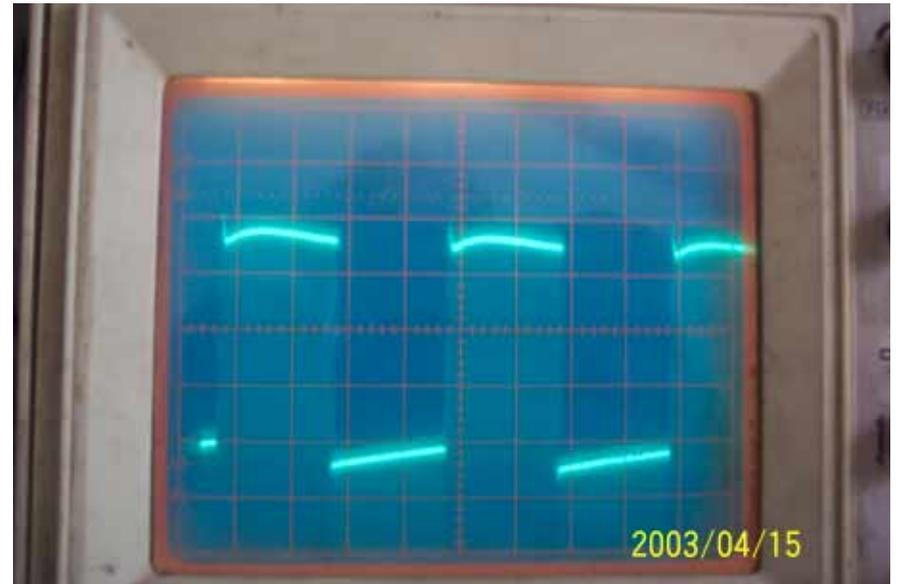
Pulse shape of the power supply of the kicker (rise-time  $35 \mu\text{s}$ ).
