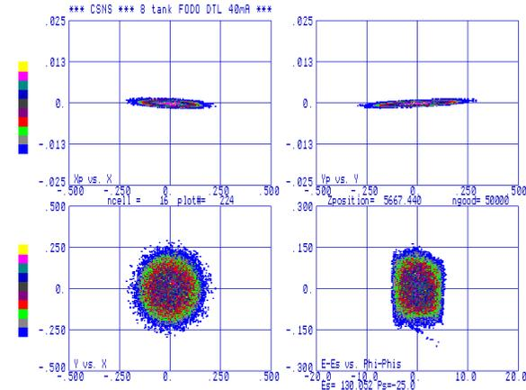
**The beam is well matched with a FODO lattice, almost no halo generation. The beam radius (Max & rms) is much smaller than the bore radius.**
